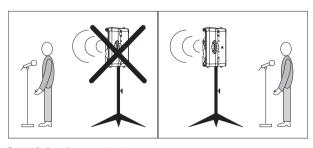
Fig. 3.2: Right and wrong positioning
